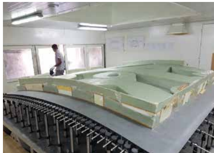
4 The final B surface laminate was applied on day three and room-temperature cured, followed by a final heated post-cure.
